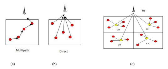
Figure 1. communication in (a) multipath (b) direct (c) LEACH
